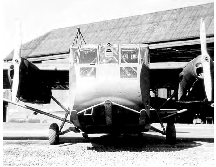
CG-4A converted to powered aircraft Burtonwood, 1945, Photo: Dick McClune Source: Aldon Ferguson
